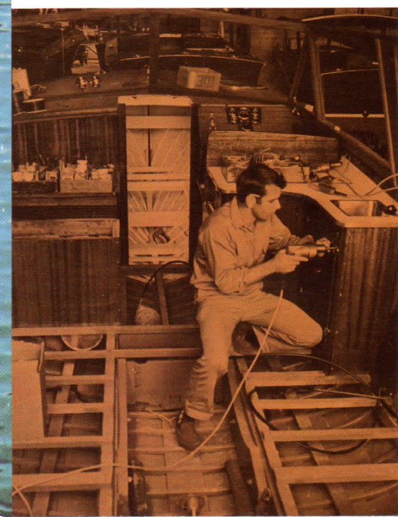
Installation (left) — final assembly of bronze-chrome hardware, engine and components, electrical wiring and accessories. This is followed by final inspection and water testing.
